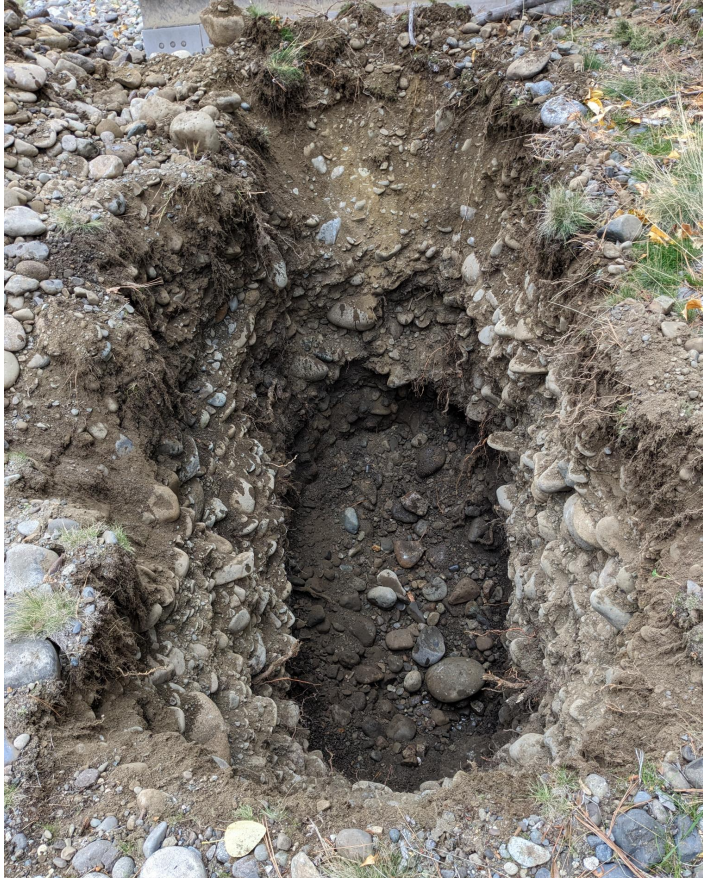
PHOTO 8: ATP-03 excavated in levee fill to 8.5 feet below ground surface.
