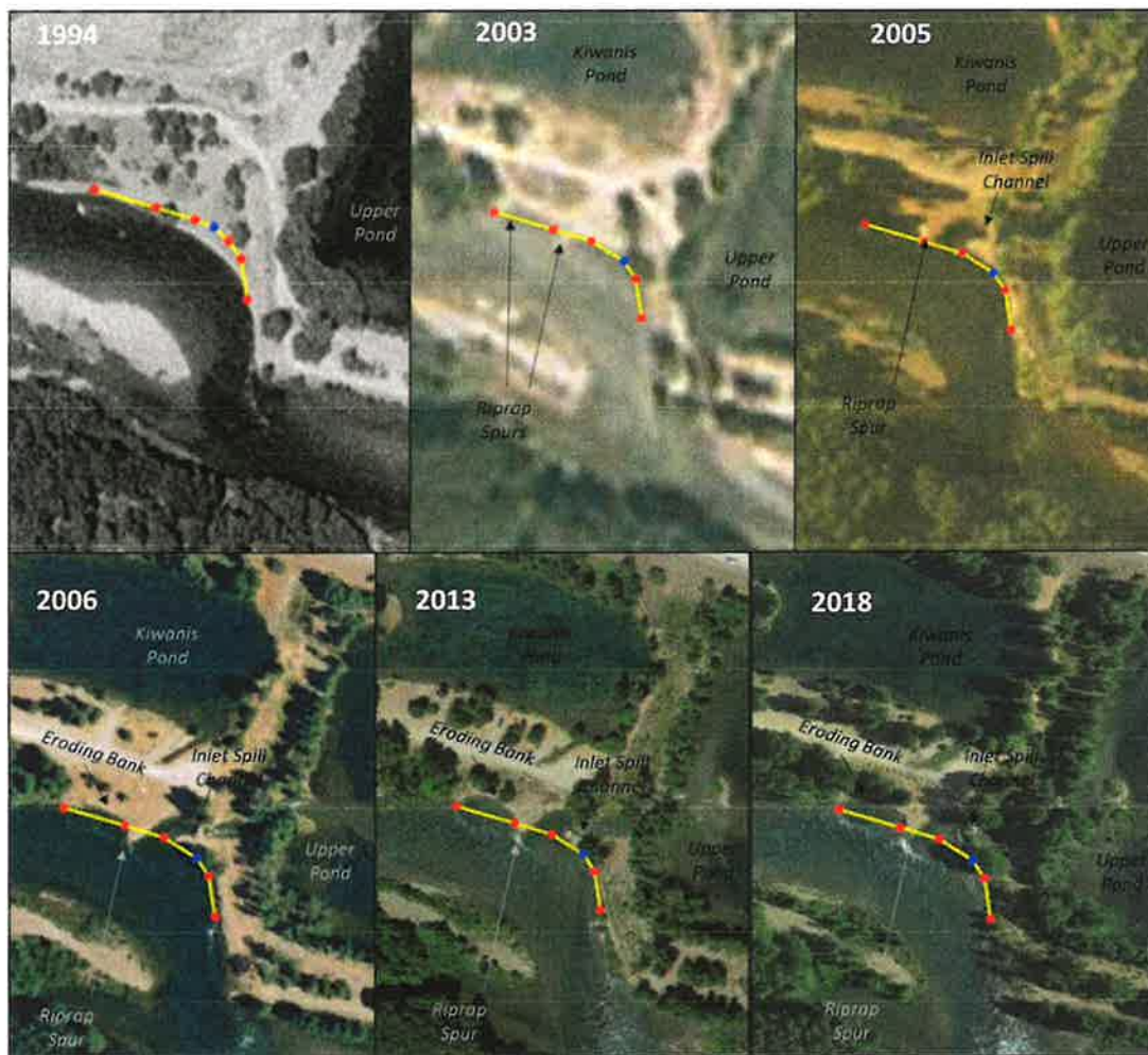
Figure 42. Sequence of aerial photos (1994, 2003, 2005, 2006, 2013, 2018). Yellow line delineates channel bank location in 2003 photo. Annotation identifies features and eroding bank of concern. (Photos: GoogleEarth)
