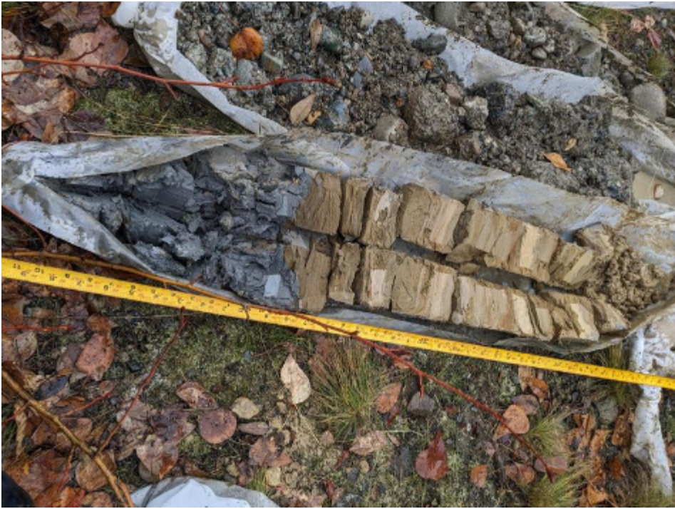
PHOTO 11: Sonic core samples from AB-06 showing transition from alluvium of the Yakima River (upper bag) to the Kittitas Drift - Indian John Subdrift Lacustrine Deposits (lower bag)
