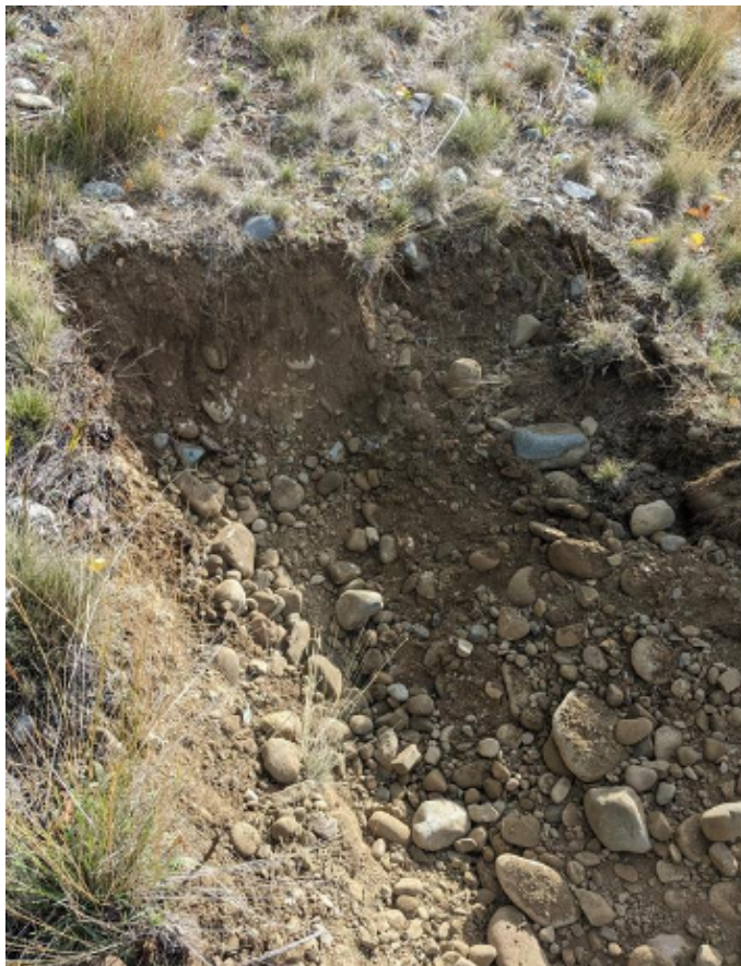
PHOTO 9: ATP-02 excavated in levee fill with thin layer of topsoil visible near surface.
