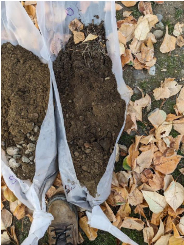
PHOTO 10: Sonic core samples from AB-02 from 0 to 2.5 feet bgs (on right) and 2.5 to 5 feet bgs (on left). Topsoil and organic material observed at surface.
